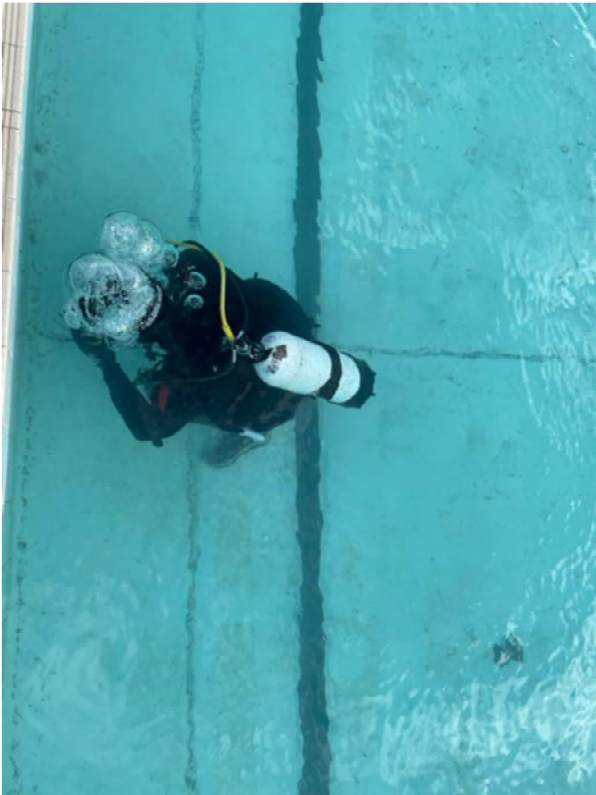
Leak testing at Walcha Memorial Baths May 2021
